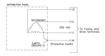
Figure 6: Earth Grounded Delta Distribution Transformer
